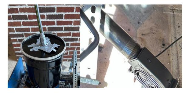
The final iteration was to use a car air conditioning fan from an old Toyota. By putting the fan into a can and having an output hole on the side, the air would suck through the top of the lid and go out through the side into a hose. This system not only worked exceptionally well to pull air through the system in a sufficient quantity, but it also led to the first successful run of the machine. That is to say that the output gas finally set on fire!
