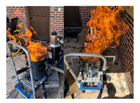
It was time to seal up the machine and turn on the fan to start running it. In a couple of minutes, the output gas would start to be able to be lit on fire and the gasifier would be working properly. In these photos, the blowtorch is off (it was used to start the fire) and the output gas burned almost indefinitely.
