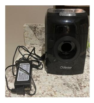
The hydrostik is like a battery—it stores the hydrogen gas to be used and converted into energy. It screws into the hydrofill in the circular area in the middle and screws into the side of the minipak.
