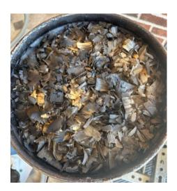
The gas is sucked up through the filter material, depositing the final bits of tar and impurities in the wood shavings before leaving the gasifier system.
