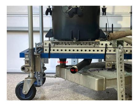
Another crucial part of the barrel is the grate basket, or where all the fuel sits during gasification. There are small, 3/8" holes drilled all throughout the basket to allow air/gas to flow through, but to not let the wooden pellets (the fuel) to fall through. The pipe on the left with the elbow attachment is the "air in" pipe. The "gas out" pipe sits under the shelf created by the basket as it helps keep any fuel from obstructing the flow of gas leaving the barrel.
