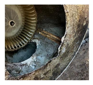
The fan was working properly, even after numerous runs of the machine—evidence that the fan was not getting caked with tar like before. However, the accumulation of tar at the beginning led to a fault in the structural strength of the fan apparatus. Originally, the fan was just attached with aluminum tape, which did not hold under the accumulation of liquid tar. The side part fell off the fan. See below.
