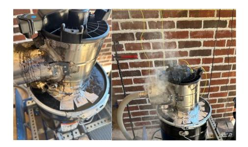
The fan seemed to solve the system's issues, but the burn was still not sustained. On to figure out how to sustain the burn indefinitely.
