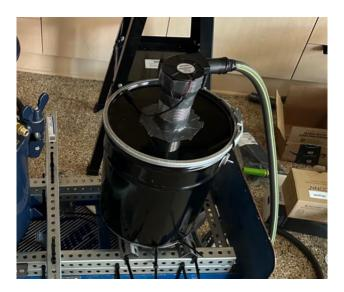
The second iteration was to use a new fan—something a little bigger and more powerful. The issue with this fan was that it sucked air through such a big area that it was hard to funnel the air to a hole the size of a hose. The fan did not suck air through the system properly. Even though it was set up to suck air out, the setup actually pushed air in the opposite direction than intended. So instead of pushing air up through the
