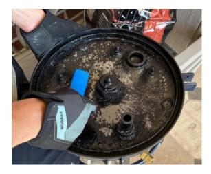
However, a larger issue is when large amounts of tar would accumulate in the moving parts, namely the fan. In the second iteration of the fan, this is what the inside of the fan looked like after a few runs:
