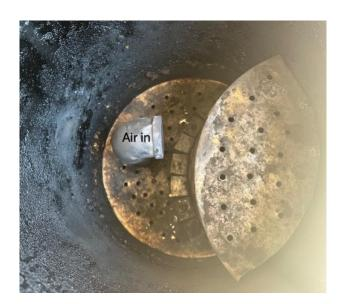
While the gasifier is running, the lid is tightly sealed—important not only for the gasification process but also important because it helps force the gas through the rest of the system (the radiator and filter bucket) and eventually to the output hose.
