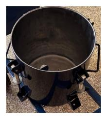
Since the barrel was an old paint mixer, there were various mixers, holes, and other devices bolted to the lid, so getting those out so they would not obstruct the fuel/basket was paramount. Since taking these devices out left holes in the lid, sealing the holes up with bolts and muffler sealer would create an airtight lid—essential for the functionality of the gasifier.
