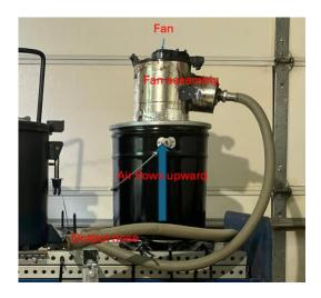
Attached to the fan is an output hose, allowing the gasifier to be connected to an engine or to just provide a singular output spot for the gas.
