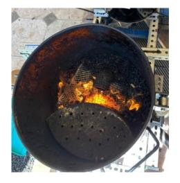
After the screen was placed, it was time to fill the machine to almost the top with new fuel (wood pellets or biomass) and let it burn until the fire became very large like so (the fire didn't need to get that large in subsequent burns):
