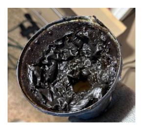
Tar accumulation to that level rendered the fan useless. A fan should not look like that—evidence that the fan or the filter was faulty. Replacing the fan for iteration 3 and 4 seemed to solve the problem as tar accumulation did not occur to the same extent as in the picture above.
