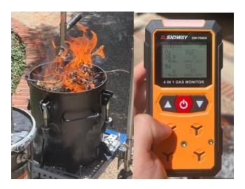
To test to see whether or not the other fuels would work, a device that measures relative quantities of gasses in the air (namely CO and  $O_2$ ) was used (right). Even though the device measures four different types of gasses, only two are part of the gasifier reactions: CO and  $O_2$ .
