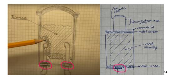
The barrel came with an inner bucket, and with a little bit of cutting with an angle grinder and drilling of holes, that inner bucket became the grate basket that goes
