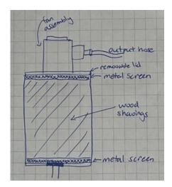
Tar is deposited around the center of the bucket more so than other areas as the center of the bucket is where most of the airflow is concentrated.
