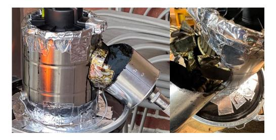
The accumulation of tar had compromised the structural integrity of the attachment, so rivets along with bent metal pieces were used to provide structural integrity to the machine and muffler sealer was used to create a strong seal. Since, the machine has held up nicely and the limited accumulation of tar has not affected the structure of the machine.
